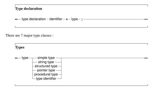
The last class, type identifier, is just a means to give another name to a type. This presents a way to make types platform independent, by only using these types, and then defining these types for each platform individually. The programmer that uses these units doesn't have to worry about type size and so on. It also allows to use shortcut names for fully qualified type names. e.g. define system.longint as Olongint and then redefine longint.
