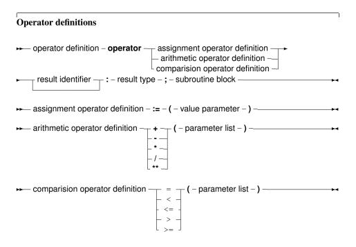
The parameter list for a comparision operator or an arithmetic operator must always contain 2 parameters. The result type of the comparision operator must be Boolean.
