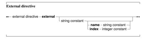
It replaces, in effect, the function or procedure code block. As an example:
