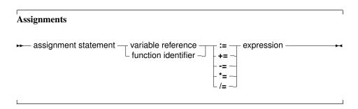
In addition to the standard Pascal assignment operator (:=), which simply replaces the value of the variable with the value resulting from the expression on the right of the := operator, Free Pascal supports some c-style constructions. All available constructs are listed in table (9.1). For these
