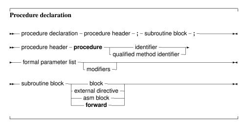
See section 10.3, page 89 for the list of parameters. A procedure declaration that is followed by a block implements the action of the procedure in that block. The following is a valid procedure:
