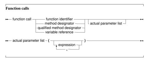
The variable reference must be a procedural type variable reference. A method designator can only be used inside the method of an object. A qualified method designator can be used outside object methods too. The function that will get called is the function with a declared parameter list that matches the actual parameter list. This means that
