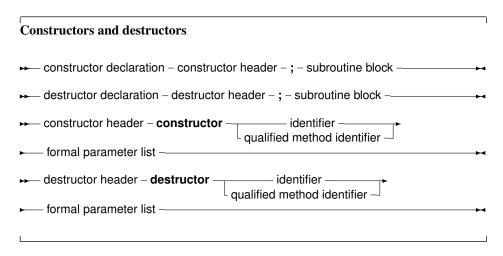
A constructor/destructor pair is *required* if the object uses virtual methods. In the declaration of the object type, a simple identifier should be used for the name of the constuctor or destructor. When
