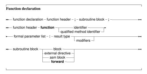
The result type of a function can be any previously declared type. contrary to Turbo pascal, where only simple types could be returned.
