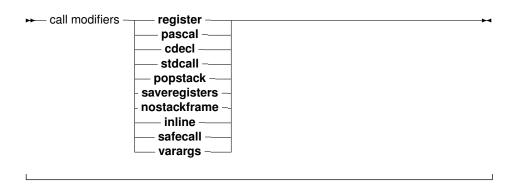
Free Pascal doesn't support all Turbo Pascal modifiers, but does support a number of additional modifiers. They are used mainly for assembler and reference to C object files.
