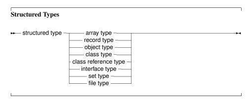
Unlike Delphi, Free Pascal does not support the keyword Packed for all structured types, as can be seen in the syntax diagram. It will be mentioned when a type supports the packed keyword. In the following, each of the possible structured types is discussed.
