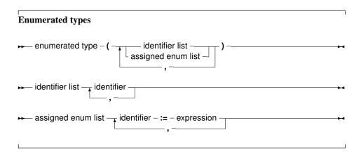
(see chapter 8, page 68 for how to use expressions) When using assigned enumerated types, the assigned elements must be in ascending numerical order in the list, or the compiler will complain. The expressions used in assigned enumerated elements must be known at compile time. So the following is a correct enumerated type declaration:
