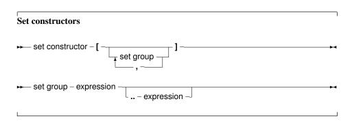
All set groups and set elements must be of the same ordinal type. The empty set is denoted by [], and it can be assigned to any type of set. A set group with a range [A..Z] makes all values in the range a set element. If the first range specifier has a bigger ordinal value than the second the set is empty, e.g., [Z..A] denotes an empty set. The following are valid set constructors:
