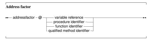
The @ operator returns a typed pointer if the T switch is on. If the T switch is off then the address operator returns an untyped pointer, which is assignment compatible with all pointer types. The type of the pointer is T, where T is the type of the variable reference. For example, the following will compile
