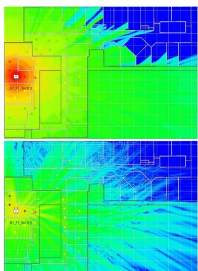
The best signal level prediction result with resolution set at 0.1m is shown on the left figure. The top plot is from the IRLA model and the bottom one is from the MR-FDPF model. The measurement points are also in this figure.
